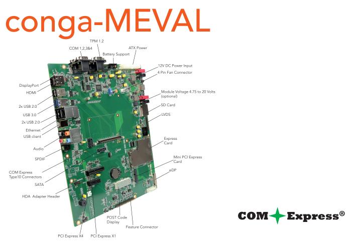
Evaluation Carrier Board for COM Express® Mini Type 10 modules. To achieve a quick start with COM Express® congatec offers an evaluation carrier board, which routes all the COM Express® signals to standard interface connectors. Supports COM Express® Mini Type 10.
